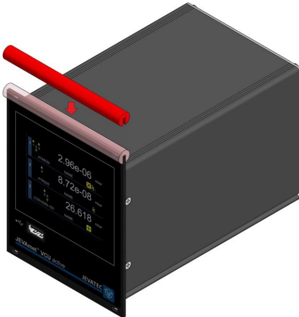
Figure 4 – Preparing the top side of the instrument for utilisation as a benchtop unit
