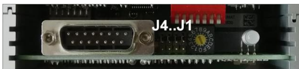
Figure 15 – Jumper for setting the operating parameters with cover plate removed
