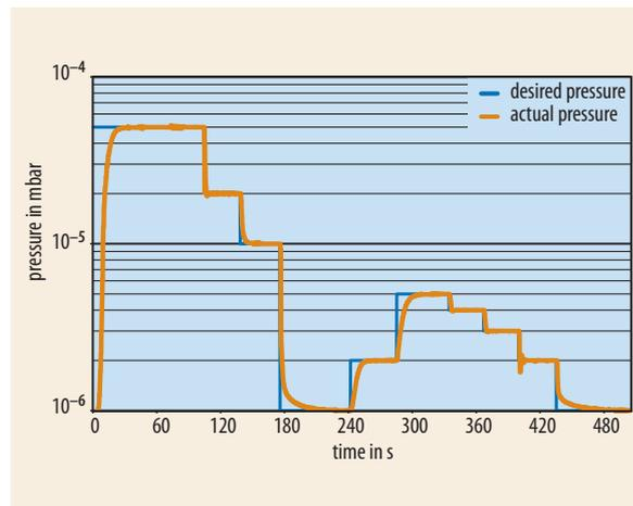
Fig. 4 Test series: stability of arbitrary pressures in high vacuum.
